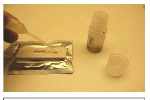
6. Draw up apple solution from the buffer bottle and pipette 2-3 drops into the well on the LFD test device. The C line should show blue. If a blue T line then appears within 10 mins the test is positive.
